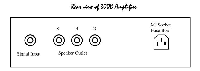
**The IEC AC power** input socket connection is located at the far left in the back. A main fuse is located inside under IEC socket. A pair of Computer grade main cables (Detachable) is included with the 300B mono-block tube amplifier. If you choose to replace the AC main cable with an esoteric type, make sure that is has a third pin for grounding the unit.
